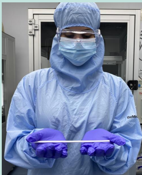
Maria Smith holding a hollow electrospun tube for vascular applications in our cleanroom
