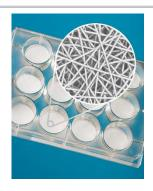
Scaffold discs in the wells are removable, held in place by retaining rings and can be taken out for imaging purposes.
